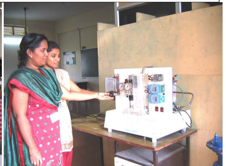
Cascade control system in P.D.C. Lab
